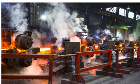
(a) A steel slab passes through several rolling stands in the hot-rolling process (Board & Vellum, 2015)
