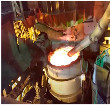
(a) Ladle of molten steel tapped from electric arc furnace (Roy, 2018)
