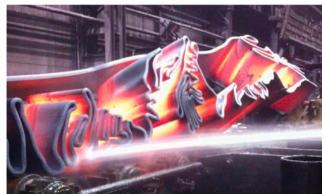
(b) A cobble resulting from a mismatch in roll force, gauge, and speed between rolling stands (Industrial History, 2021)
