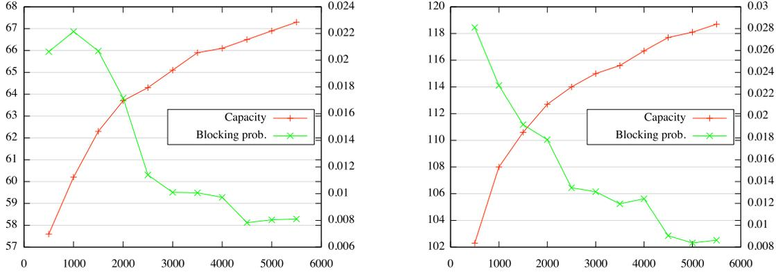
Figure 2: Resulting objective functions and blocking probabilities for Formulation 3 with  $\gamma = 0$  on Ring topologies with 7 and 9 nodes with homogeneous traffic load  $\rho = 0.2$  for different sample sizes.
