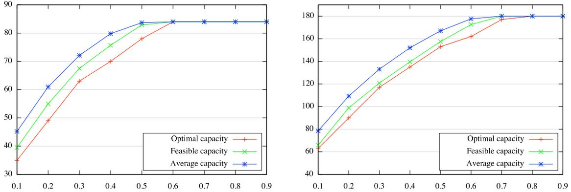
Figure 3: Resulting objective functions for Formulation 3 with  $\gamma = 0$  on Ring topologies with 7 and 9 nodes for different homogeneous traffic loads. ( $|S| = 500$ )
