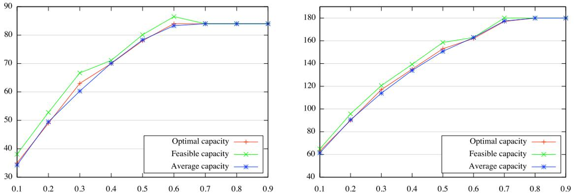
Figure 4: Resulting objective functions for Formulation 3 with  $\gamma = \alpha$  on Ring topologies with 7 and 9 nodes for different homogeneous traffic loads. ( $|S| = 500$ )
