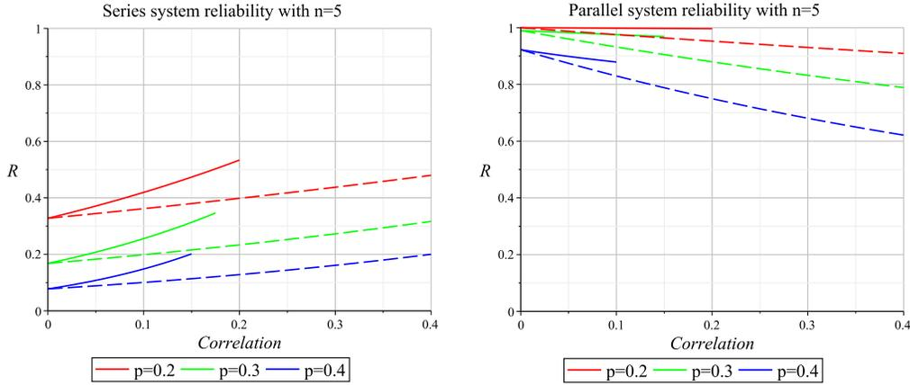
Figure 1: Reliabilities of series and parallel networks with  $n = 5$  components, as functions of the correlation between any pair of link states, for various values of the elementary reliability  $p$  and for two choices of copulas: either only copulas of size  $\leq 2$  or only copulas of size 1 or  $n$  (all components).
