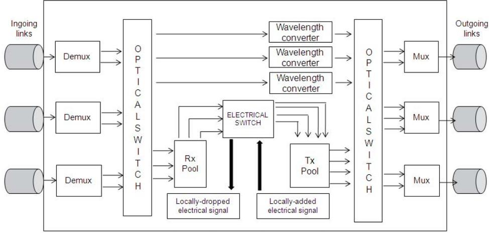
Fig. 1. Diagram of WDM node
