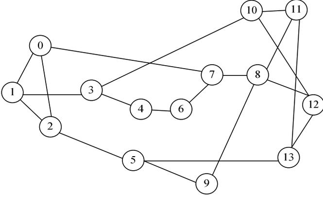
Fig. 2. NSFNet (14 nodes, 42 unidirectional links).
